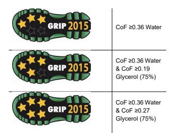
Not all workplaces will require 5-Star footwear to prevent slips. For environments where water is the only likely contaminant, 2- or 3-Star footwear should significantly reduce slip risk. 4- and 5-Star footwear is only needed where more viscous contaminants, such as oil, are present (e.g. in kitchens).
