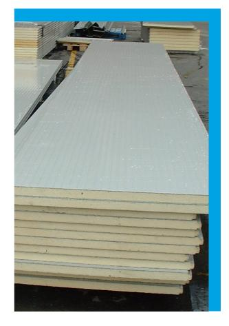
There have been numerous serious fires over the years, where FISP panels have been used in construction, resulting in significant loss of facilities and resultant business interruption consequences. The main detracting features of using a combustible or nonapproved sandwich panels are as follows:
