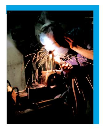
For hot work that cannot be carried out in a designated workshop, additional procedures will be required controlled by an effective hot work permit.
