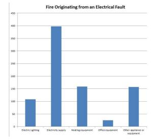
Whilst it is not possible to separate out losses specific to portable electrical appliances it is clear that faulty portable electrical appliances are a major cause of fires and that adequate measures need to be taken to prevent or mitigate the risk they present.
